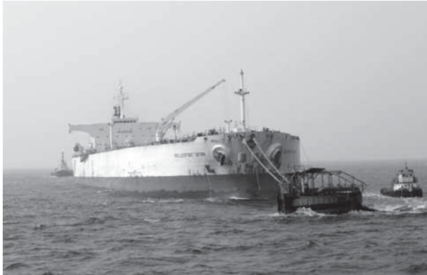
Crude Carrier discharging into IndianOil SPM
